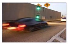
"real-time" traffic conditions and cycle times will be adjusted to control traffic at that moment. Traffic sensors in the pavement indicate how heavy traffic volumes are on the highway. Lighter volumes will typically speed up the red-green cycle to let more cars enter the expressway. Similarly, if the sensors detect heavier traffic on the highway, the red-green cycles would be adjusted to space out merging traffic.
