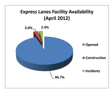
The entire 95 Express lanes (both directions) were open to motorists 94.7% of the time, while closed 3.0% due to 9 planned construction/maintenance events (each lasting 4 hours, 45 minutes in duration on average) and 2.4% due to 154 non-recurring events (each lasting approximately 13 minutes in duration on average).
