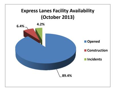
The entire 95 Express lanes (both directions) were open to motorists 89.4% of the time, while closed 6.4% due to 18 planned construction/maintenance events (each lasting approximately 5 hours, 18 minutes in duration, on average) and 4.2% due to 190 non-recurring events (each lasting approximately 19.5 minutes in duration, on average).
