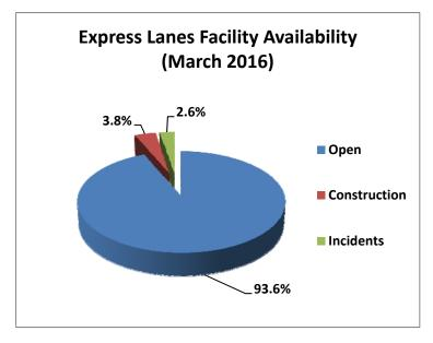
The entire 95 Express lanes (both directions) were open to motorists 93.6% of the time, while closed 3.8% due to 14 planned construction/ maintenance events (each lasting approximately 4 hours, 0 minutes in duration, on average) and 2.6% due to 95 non-recurring events (each lasting approximately 25 minutes in duration, on average).
